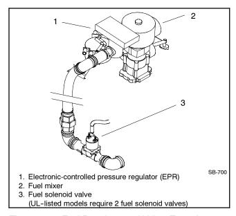
Figure 3-8 Fuel Regulator and Valve, Typical
